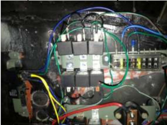
**Relays and fuse box in place and starting to get wires. I moved all the electrical system components on the inside of the firewall**
