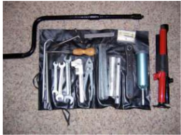
Original tool kit with crank, wheel brace and jack
