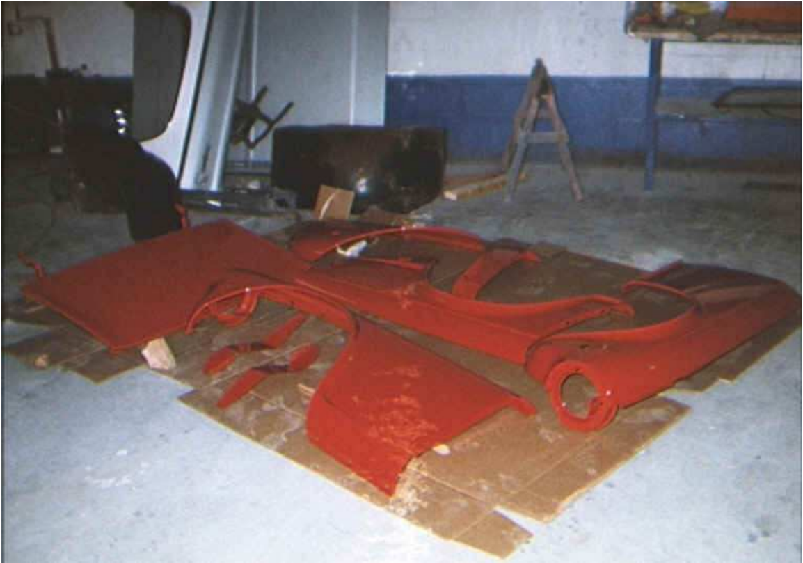
Body panels prime and painted.
