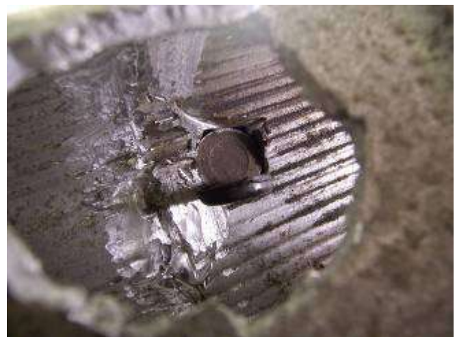
The U-Joint bearing cap embedded in the other side of the trailing arm as seem though one of the holes. Wonderful
