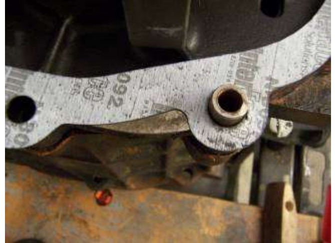
The one place where the rear cover gasket didn't cover all the metal, but enough to work
