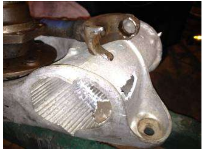
Holes in the trailing arm & busted yoke
