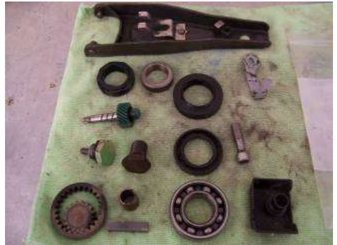
Left-over/replaced parts after trannie was repaired.
