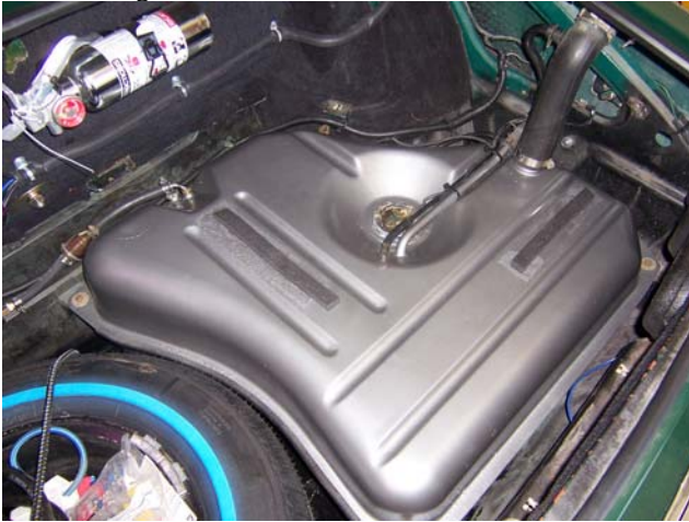
The Fixed Gas Tank In The Stag – I Knew I Had A Picture Somewhere!
