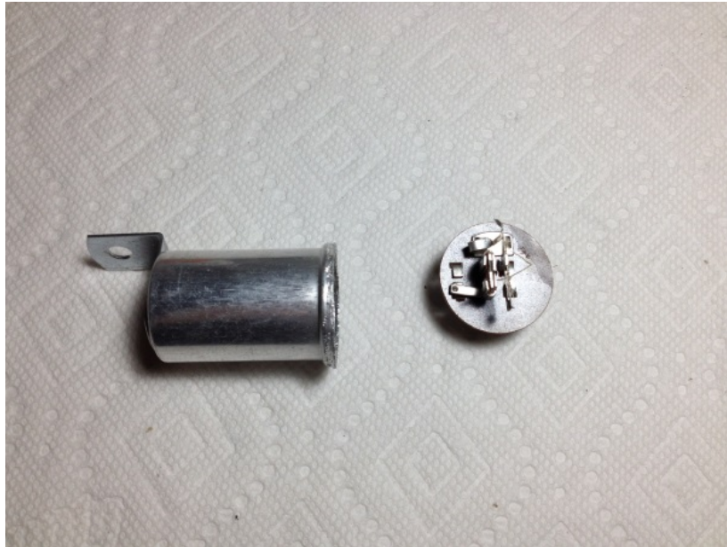
Figure 3 – Yep, that’s all that is inside the original-style flasher
