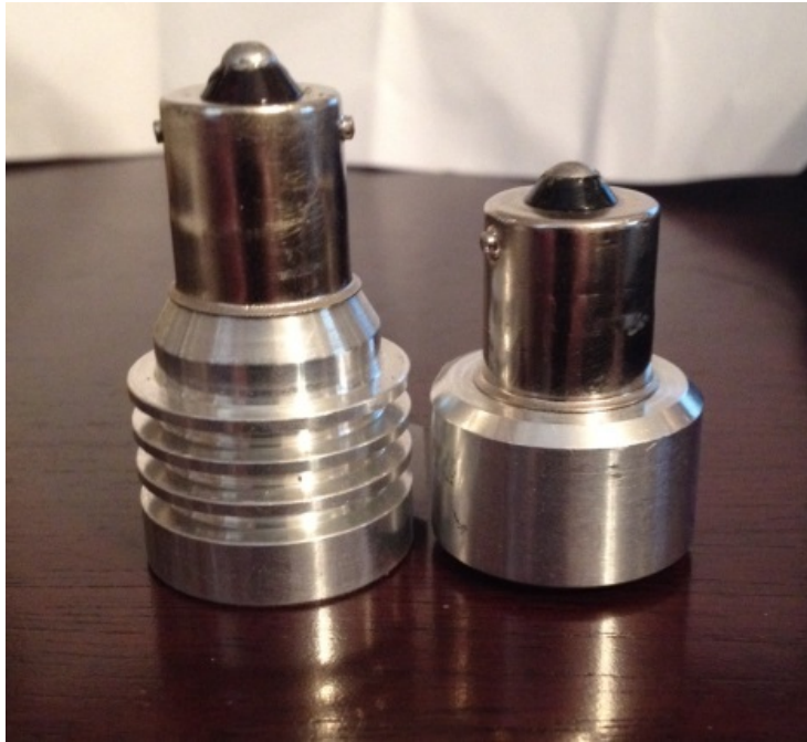
Figure 8 – Difference between the standard LED designed to fit a 1156 socket (and with a dual filament the 1157) on the left and the shorter one required for turn signal applications on my TR3A
