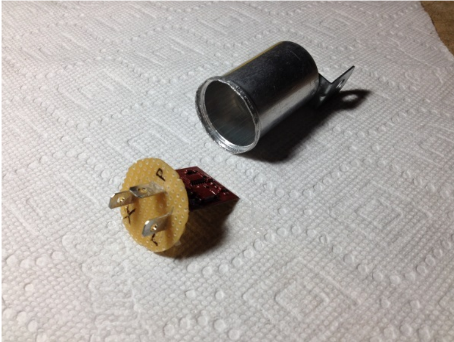
Figure 5 – Ready to put back together – just crimp the board back into the bottom of the canister
