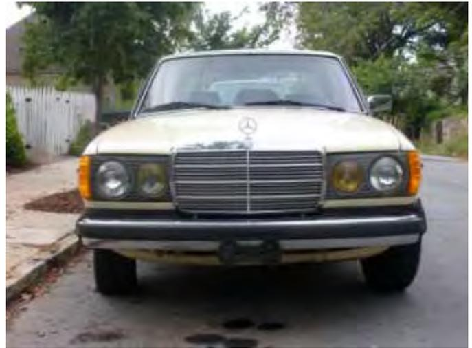
Turns out that body style used 5.75" fog lights that will fit where the original high-beam-only inner lights were. So, where do I find those lights?
