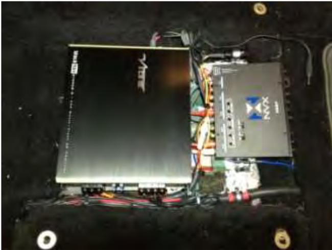
I had to cut back the carpet a bit (it's sad carpet anyway) and take the end pieces off the amp, but it fits – snugly. Power amp is to the left, pre-amp to right, and you maybe can just make out the USB power adaptor at the top right.
