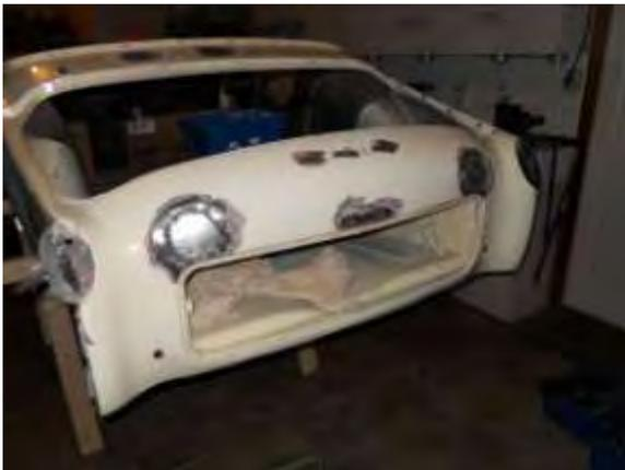
**Rear apron with turn signal mounts taken out – another job for epoxy and counter-sunk pop rivets!**
