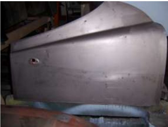
Dip line on passenger's door
