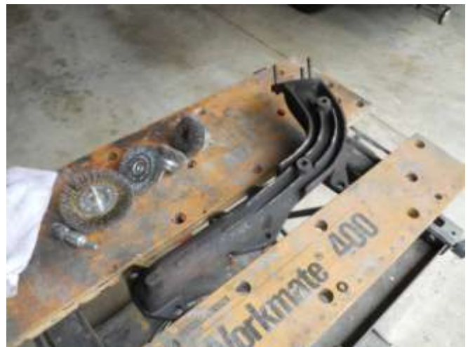
Rust off, ready for first coat
