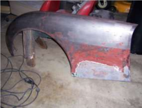
Dip line showing on driver's fender – paint sticks much better where it was dipped
