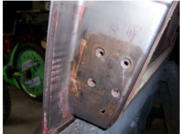
Crack on the outside of the hinge mount, passenger door
