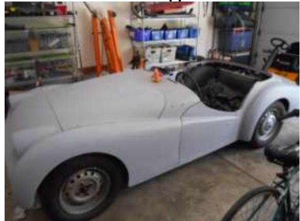
Stripped body back on the frame to test fit and fix alignment issues
