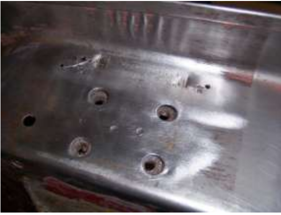
Stop-drilled cracks on the driver's side door I have my appendages crossed!
