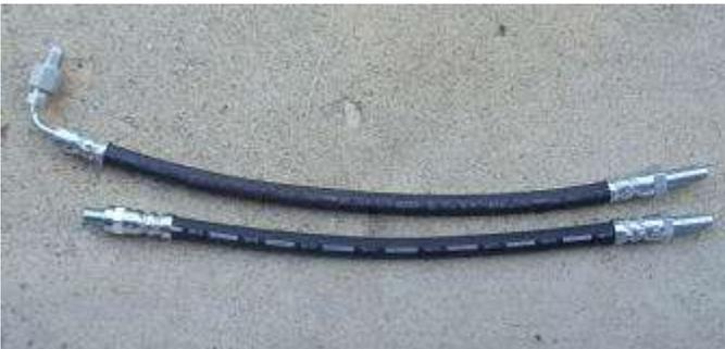
Top Hose is for Toyota caliper, Bottom Hose is standard TR.
