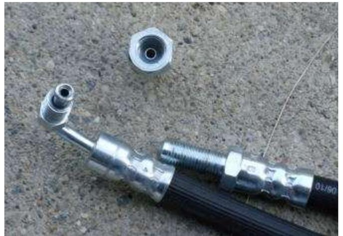
Toyota caliper hose end and SAE to Metric adapter.
