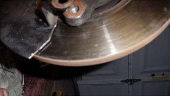
Where you cut off material from lower side of dust shield.
