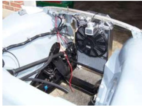
**Radiator in place – note the engine bay wiring harness along the side**
