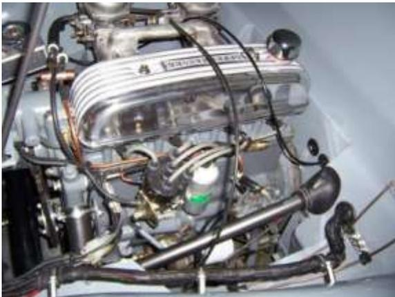
**The accelerator cable is the one in the middle.**
