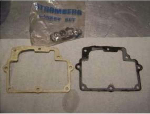
**NOS on left, Apple Hydraulics gasket on right. Picture does not give justice to how bad the Apple gasket was. Dark spots on the Apple gasket are gas-soaked areas that have not evaporated off yet. Nice...**
