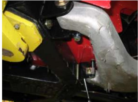
Since adjusting the camber on the rear wheels entails removing the trailing arm mounts I decided it would be well worth the cost to be able to just turn a bolt to adjust them.
