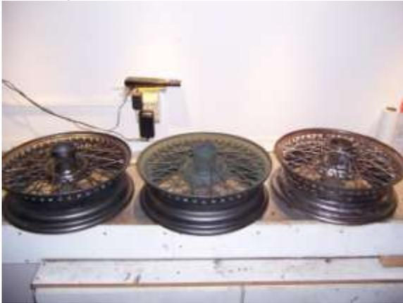
**Cleaned wheel on right, primed wheel in the middle, and finished wheel on the left**
