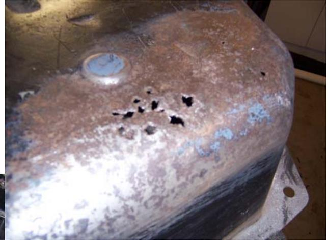
**Figure 3: Holes In The Gas Tank**
