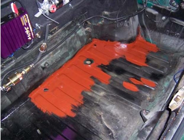
**Figure 2: Trunk Floor Being Dealt With**
