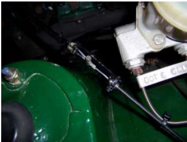
Inside cables soldered, barrel-clamped and in place
