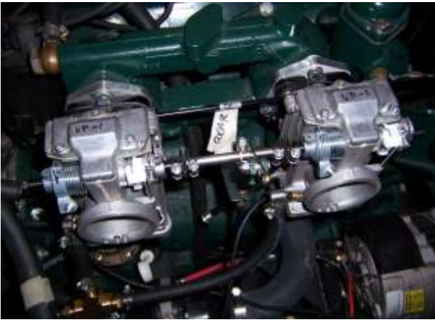
New Mikuni carbs in place on new carbs mounts
