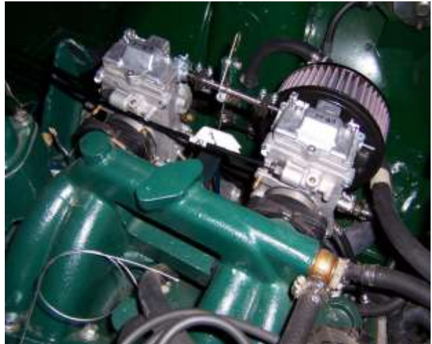
Choke cables in place – note that they have to run forward a ways before you can reverse them due to the intake manifold
