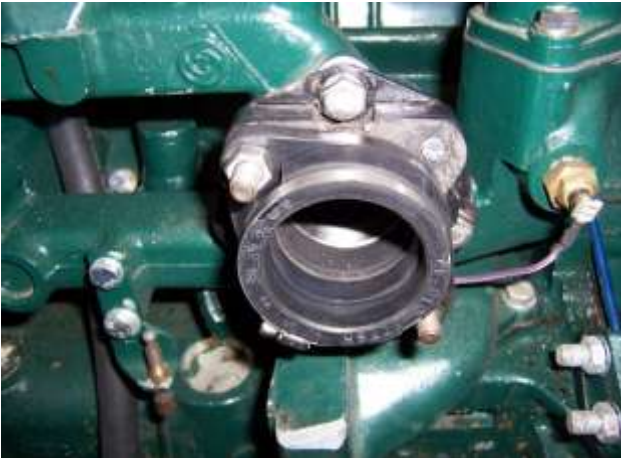
Mikuni adaptor in place on an old carb mount. Note that it only uses two of the four studs so I cut the non-used ones off
