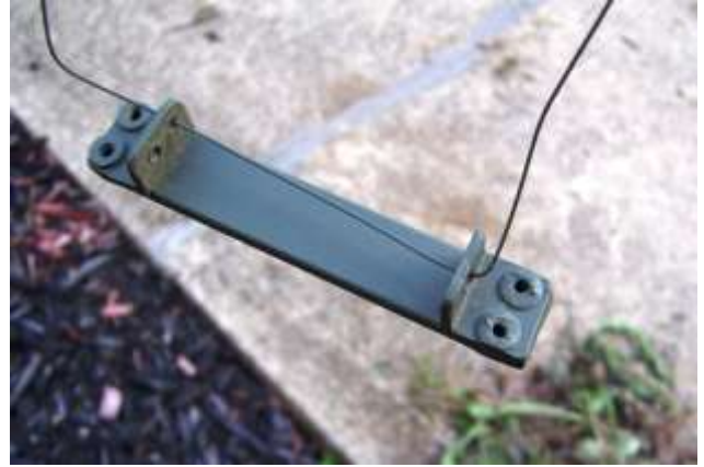
My first try at a cable junction "gizmo", the CJG, to hold the cables and transfer the compression load of choke operation
