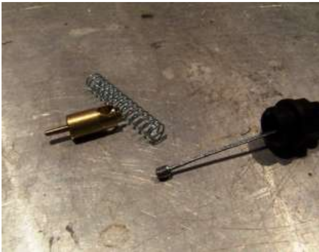
Choke valve, spring, and cable
