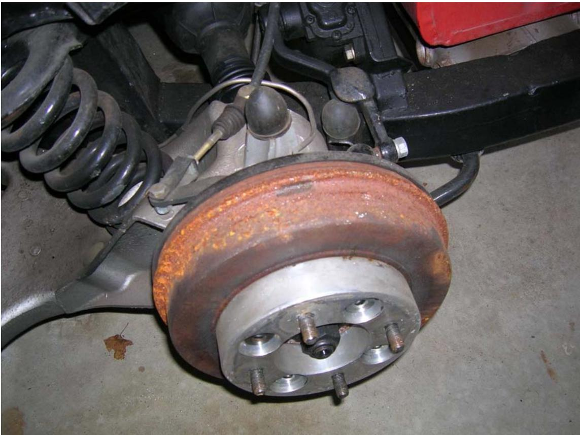
Well the best solution I could come up with was this aluminum spacer. It moved the wheel out to the proper distance when measured from the center of the car. You can still see the shock damper arm doesn't match the rubber stopper, but I had arm bent to lineup correctly with the trailing arm. Not pretty, but it has solved the problem. Over the years, I found a good spare frame that I have thoughts of changing out sometime in the future.
