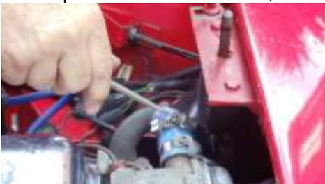
Bruce's method of two clamps, one on either side of tape over tear in hose.
